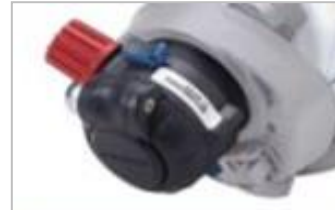
The compact supply valve does not obstruct the view and the double locking device prevents improper detachment, and in case of an emergency, the supply valve can be removed with one hand (central purge button for additional supply)
